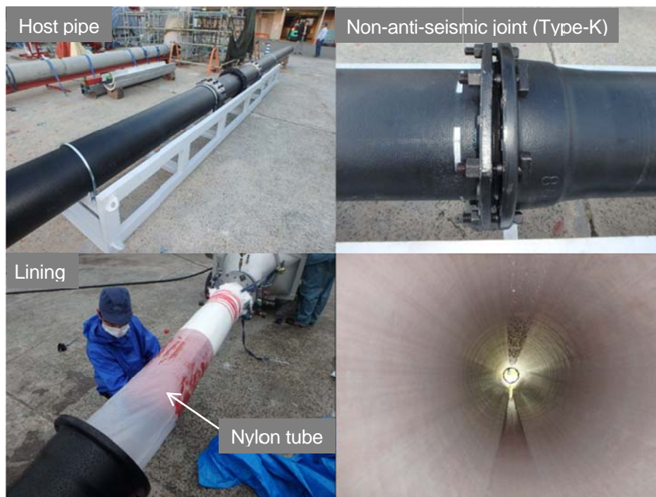
Figure 6. Stages of specimen preparation
